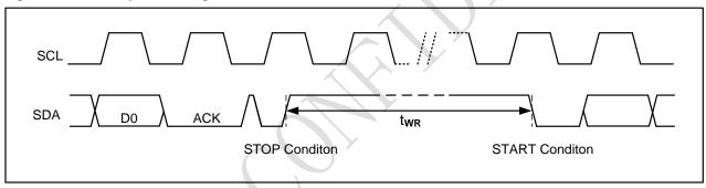
Note: [1] The write cycle time t<sub>WR</sub> is the time from a valid stop condition of a write sequence to the end of the internal clear/write cycle.
