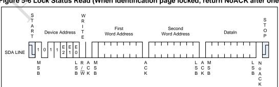
Figure 5-6 Lock Status Read (When Identification page locked, return NoACK after one data byte)
