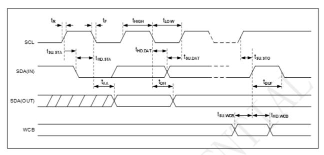
**Figure 3-2 Write Cycle Timing**
